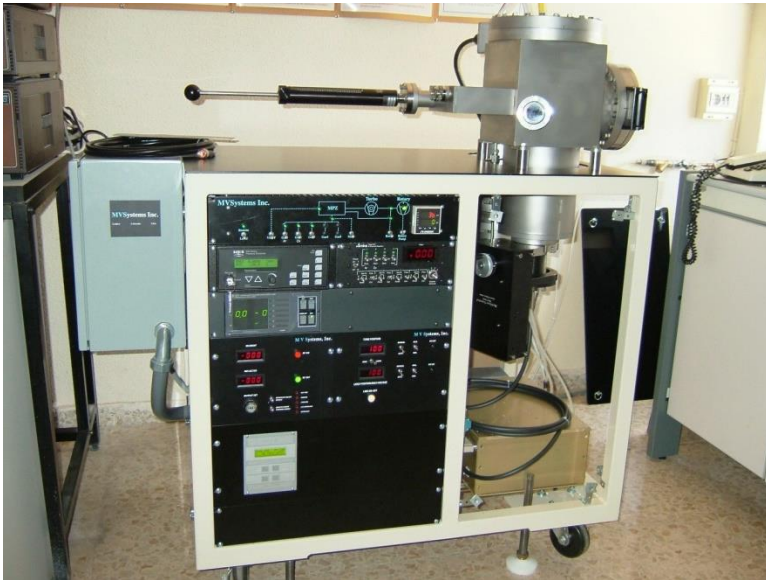
Figure 3: Photography of the physical deposition system used for the \text{Cu}_3\text{N} thin film fabrication.
