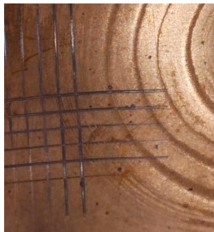
Figure 5: Photograph of a PEEK-copper composite made by chemical plating, after cross-hatch and peel test.
