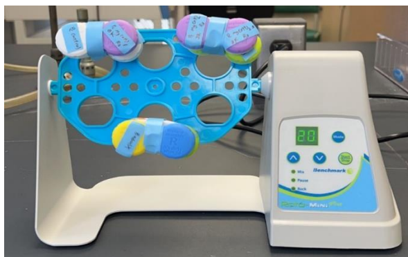
Figure 5: The pods were attached with tape to the mini rotator device for consistent agitation of the bacterial broth and surface renewal of the disks inside the pods. The blue tray holding the pods rotates around the horizontal axis.
