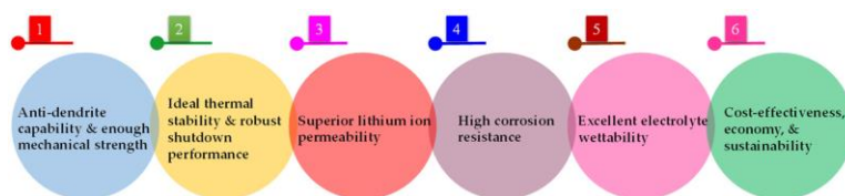
Figure 2: Schematic illustration of separator performance requirements to consider when selecting the appropriate separator for rechargeable LIBs.
