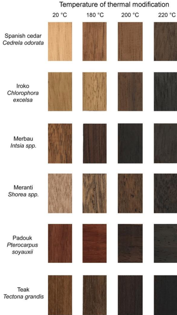
Figure 1: The appearance of reference and thermally modified samples at temperatures of 180, 200, and 220 °C.
