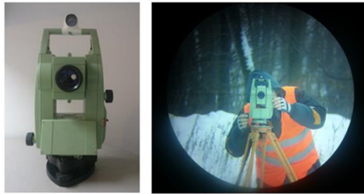
Figure 11: Changing the total station by mounting a mini prism.
