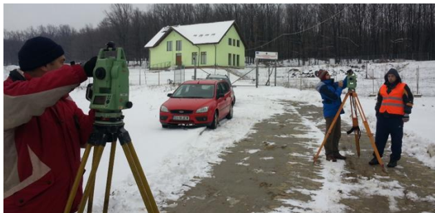
Figure 12 (Foto and scheme): Determination of the two mounted mini prisms constants (foto).
