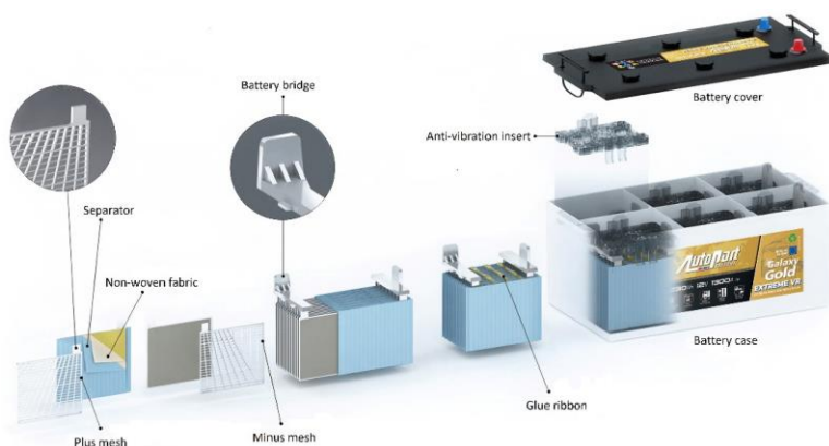
Figure 1: Battery construction diagram (produced by AUTOPART-Mielec, Poland).
