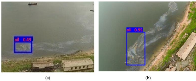
Figure 10: Detection: (a) spot detection at an observation angle of about 45^\circ ; (b) probability of detection when a slick is located directly under the drone camera (nadir).
