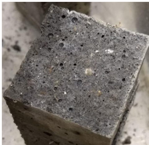
Figure 6: Cement mortar samples with 0.5% E. globulus bark fibres.
