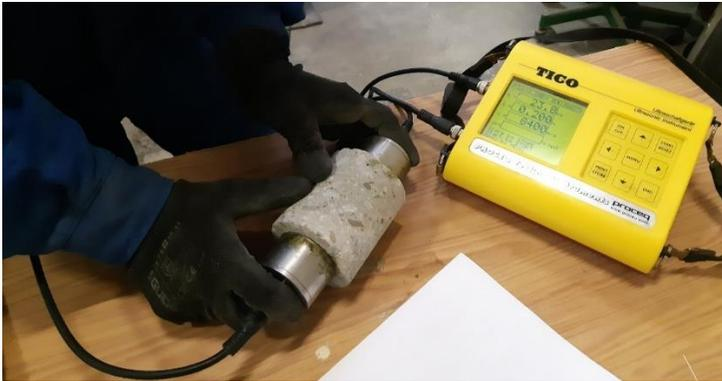
**Figure 2:** UPV testing.
