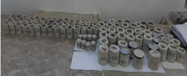
**Figure 1:** Concrete core specimens.
