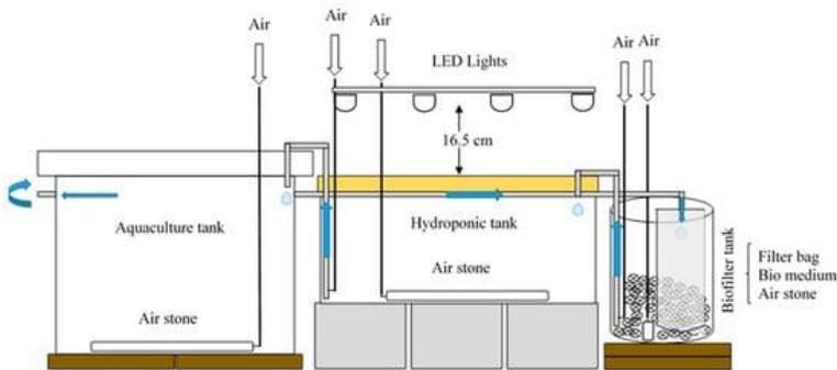
**Figure 1:** Schematic diagram of an aquaponic system unit.
