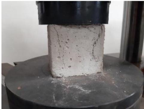
(c) Compressive strength test set-up
