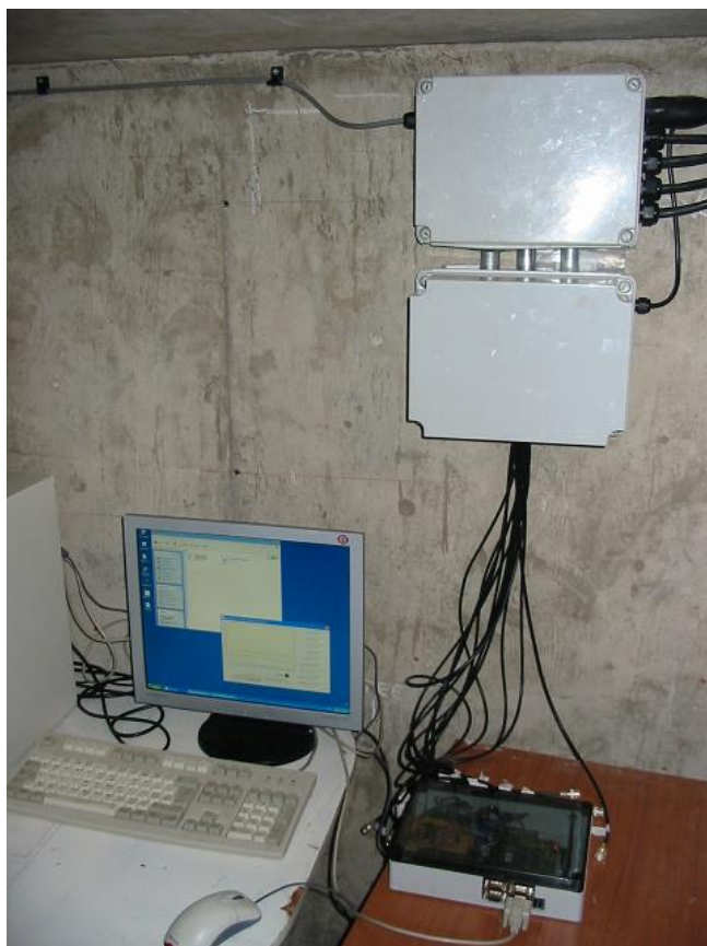
Figure 14: Device implementation in IP67 enclosure (bottom right), interface to local PC (bottom left) and instrumentation/communication interfaces (top right).
