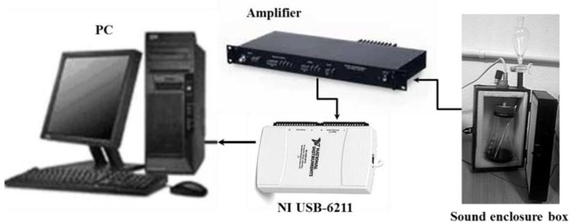
**Figure 2:** Scheme of the experimental set-up for acoustic emission analysis [13].
