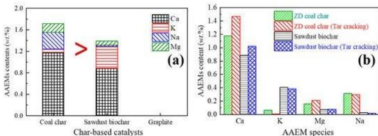
**Figure 2:** Alkali and alkaline earth metal species (AAEMs) contents in char-based catalysts: (a) Raw and (b) changes before/after tar reforming.
