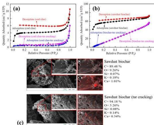
**Figure 4:** Physical characteristics of char-based catalysts on in-situ biomass tar reforming: Isothermal nitrogen adsorption/desorption curves of (a) coal char and (b) sawdust biochar; (c) SEM-EDS results of sawdust biochar.
