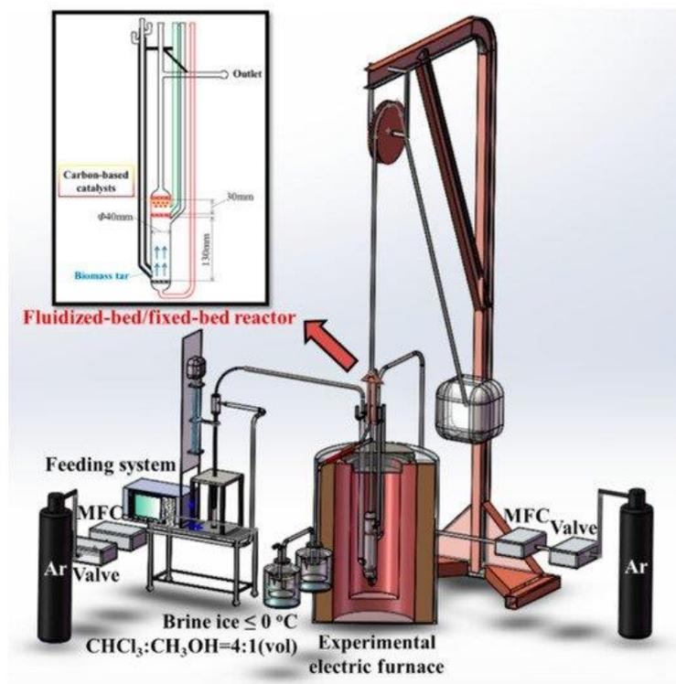
**Figure 6:** Experimental system of fixed-bed/fluidized-bed reactor.
