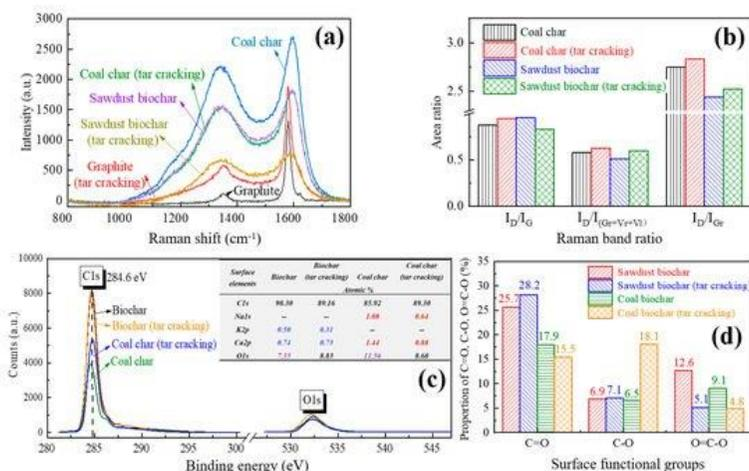
**Figure 3:** Chemical characteristics of char-based catalysts on in-situ biomass tar reforming: (a) Raman spectra; (b) Raman band ratio; (c) C1s and O1s peaks in XPS spectra; and (d) Proportion of C=O, C-O, O=C-O functional groups.
