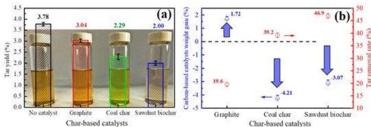
**Figure 1:** In-situ biomass tar reforming results over char-based catalysts: (a) Tar yields, and (b) weight gain and tar reforming rate for the char-based catalysts.
