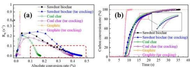
**Figure 5:** Reactivity analysis of char-based catalysts on in-situ biomass tar reforming from a micro fluidized bed reaction analyzer (MFBR–MR): (a) Reaction rate versus absolute carbon conversion rate and (b) carbon conversion rate with time.
