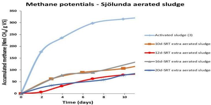
**Figure 3:** Relation between digestion time and accumulated methane gas production related to different extra aerated Solids Retention Times (SRT) in the activated sludge reactor.
