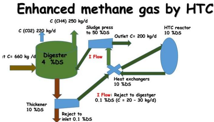
**Figure 5:** Simplified balance on the combination anaerobic digester and HTC-reactor with recycle of reject to digestion.
