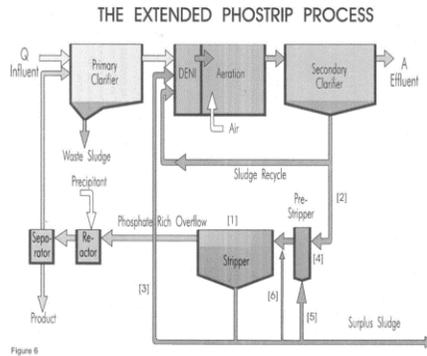
**Figure 4:** Principal flow sheet for the Phostrip Process.
